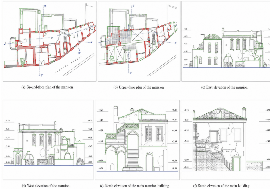
Figure 8: Plans, elevations, and three-dimensional shell-element model of the stone-masonry building
